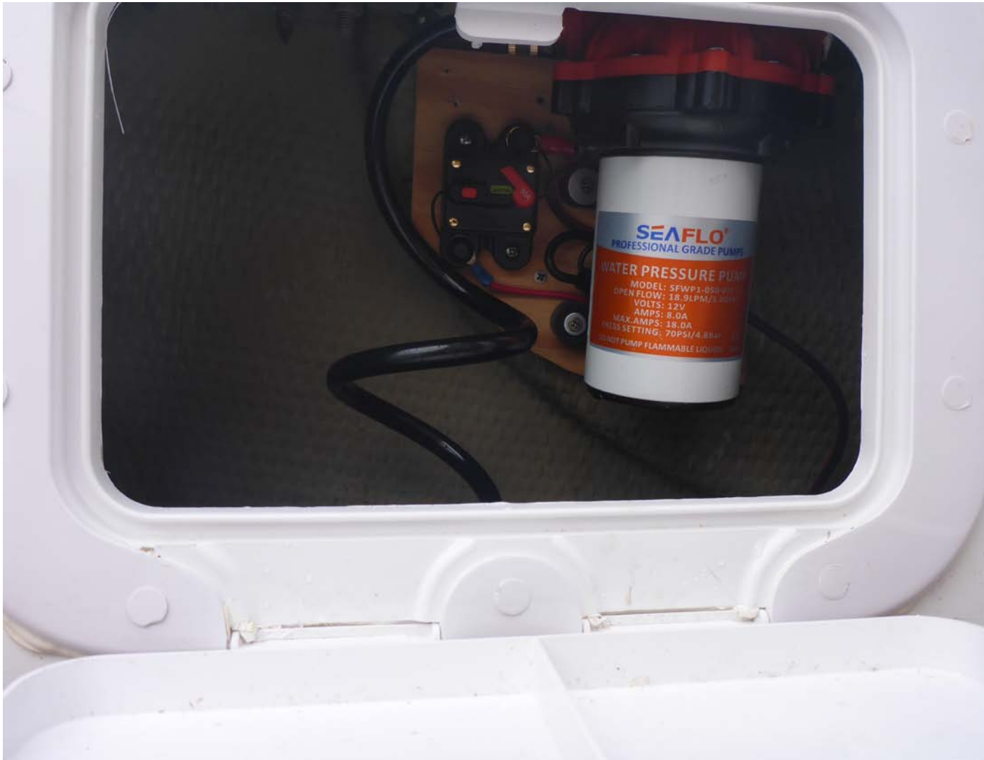
Figure 44 Pressure pump in cockpit. The switch on the automatic fuse is seen (red). Push it down to give power to the pump. The pump will start and stop when pressure has built up. Opening the valve on the end of the hose, the pump will start. It will only work well after a few seconds since air in the system has to be pumped out.
