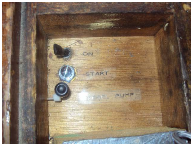
Figure 56 Emergency starting. Contact "On" will give electricity to motor independent of instrument panel. "Start" will turn the starter. "Diesel pump" will disconnect power form diesel pump when instrument panel is used. This contact has a lock which must be cut off in order to turn the switch off. CURRENTLY NOT CONNECTED.
