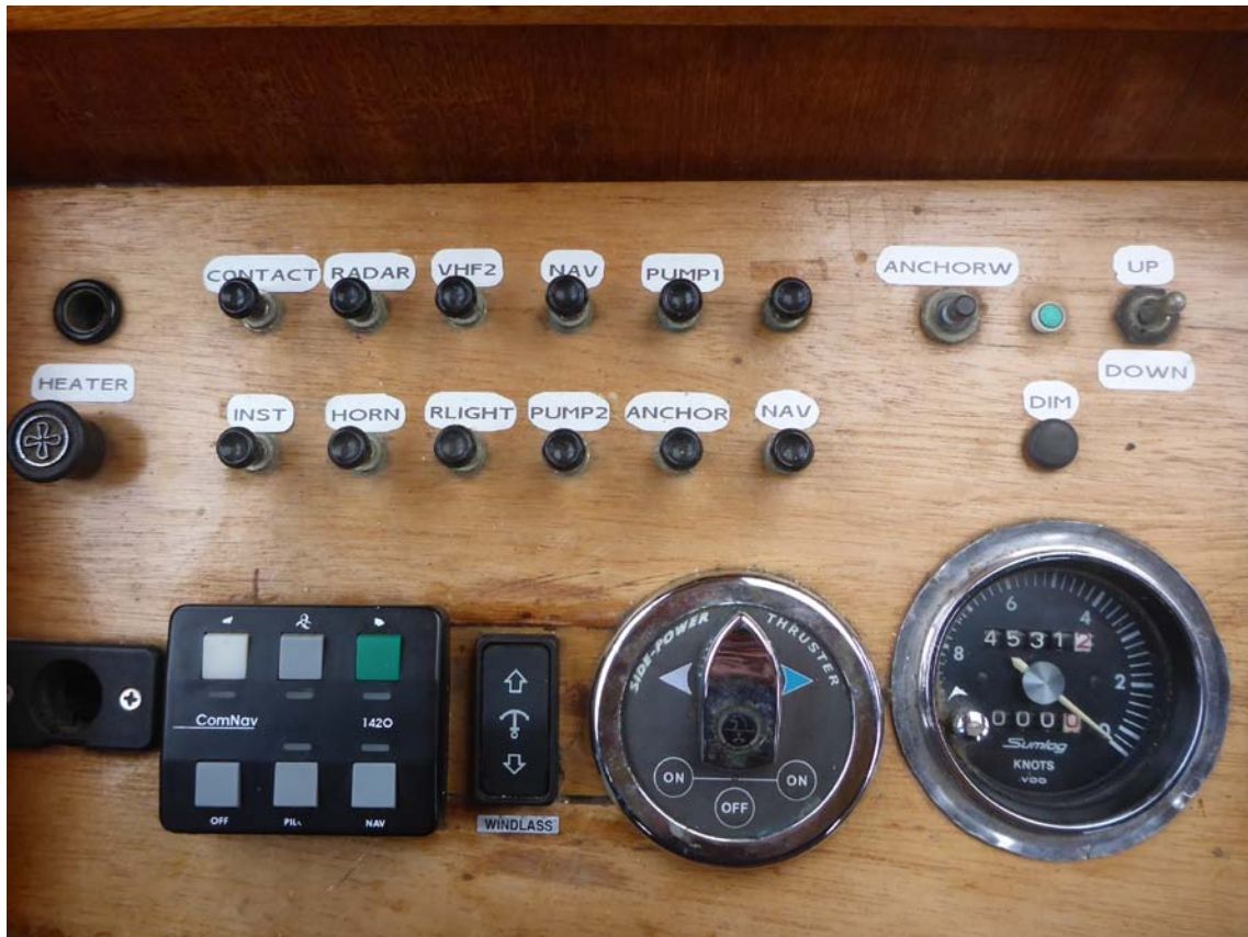
Figure 3 Left part of instrument panel. Left round switch is for heating. ComNav is the auto pilot. Above the log is seen the dimmer for the compass light. The windlass is for the front winch. The mechanical log to the right does not work, the drive cable is missing.
