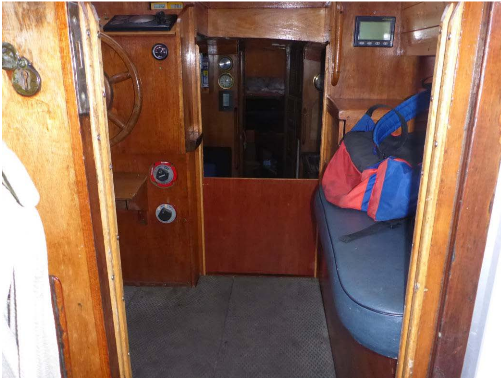
Figure 50 One of two wash boards which can be used to block off the main cabin. It is located just below the stairs. Also used for a bench, see Figure 47.
