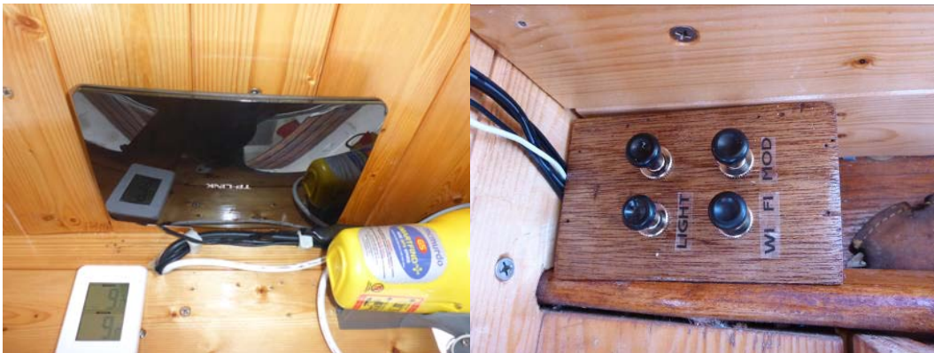
Figure 45 Left: TP Link modem and router. Right: Switch modem and outside light. WyFi is not used.
