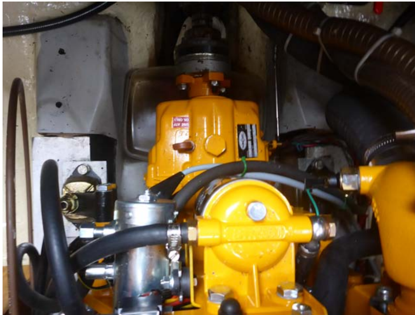
Figure 19 Gear box with dip stick (red left) and filler cap (big screw in the middle).
