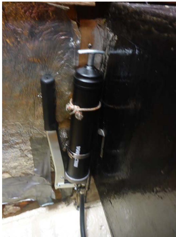
Figure 52 Middle: Access to propeller axle pack box from cargo bay. The black surface is the back of the large fuel tank. Left: Propeller axle pack box. Right: Key used to tighten the pack box.
