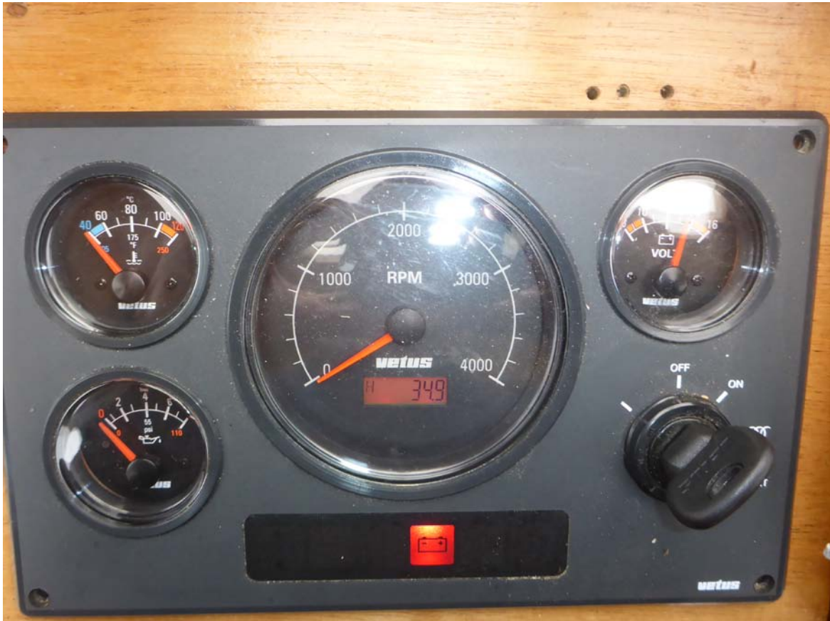
Figure 4 Motor instrument panel. When key is turned, before motor runs, only the battery light will be on. It turns off when the motor is running.
