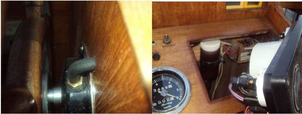
Figure 13 Left: Steering wheel and hose to the hydraulic oil reservoir. Right: Reservoir for hydraulic oil, brown bottle with white cap.
