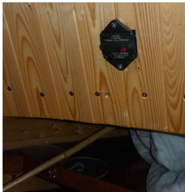
Figure 42 The automatic breaker for the front winch.
