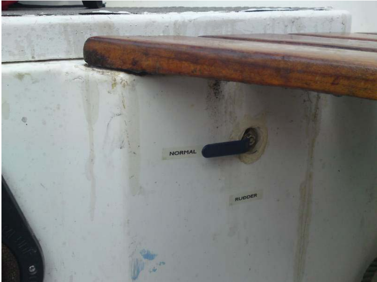
Figure 12 The handle of the bypass valve to change from tiller steering (rudder) to wheel steering (normal).
