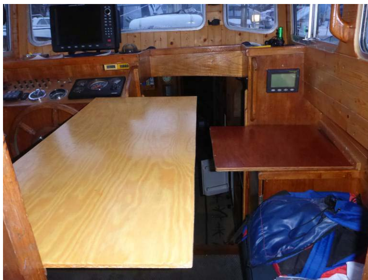
Figure 47 Table and bench using the seatback from the main cabin and the large wash board.
