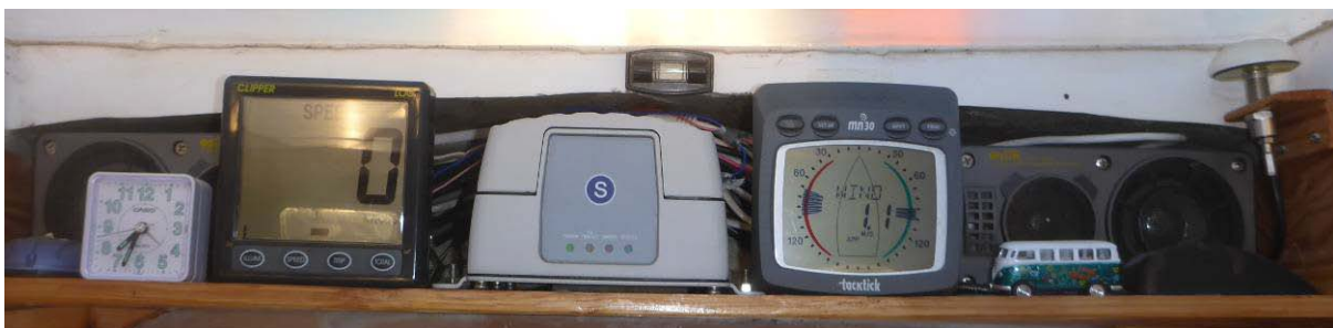
Figure 38 Instrument panel on top. Blue 'mouse' to the left is GPS for the PC. Next follows the Log. In the middle is seen the AIS. To the right of the AIS is seen the wind instrument and to the far right right is the GPS for the VHF (black) and for the AIS (white).
