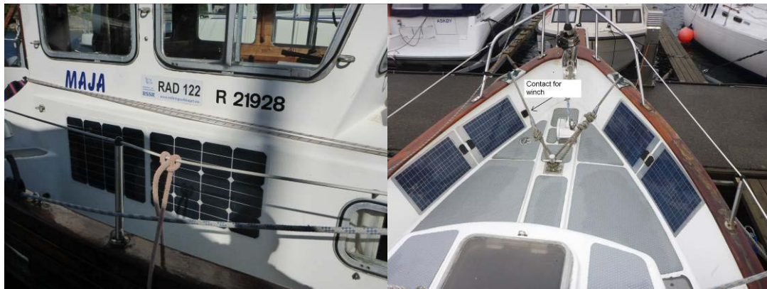
Figure 30 Right: Solar panels in the front. Note switch for front winch. Left: Solar panels on the side.
