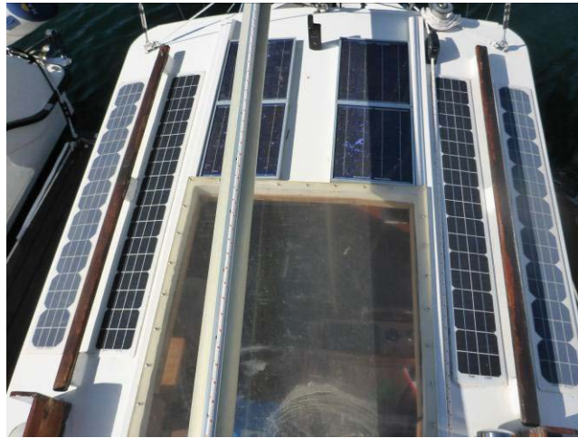
Figure 29 Solar panels on dog house roof. The long panels can be walked on, while the square panels will break if walked on.
