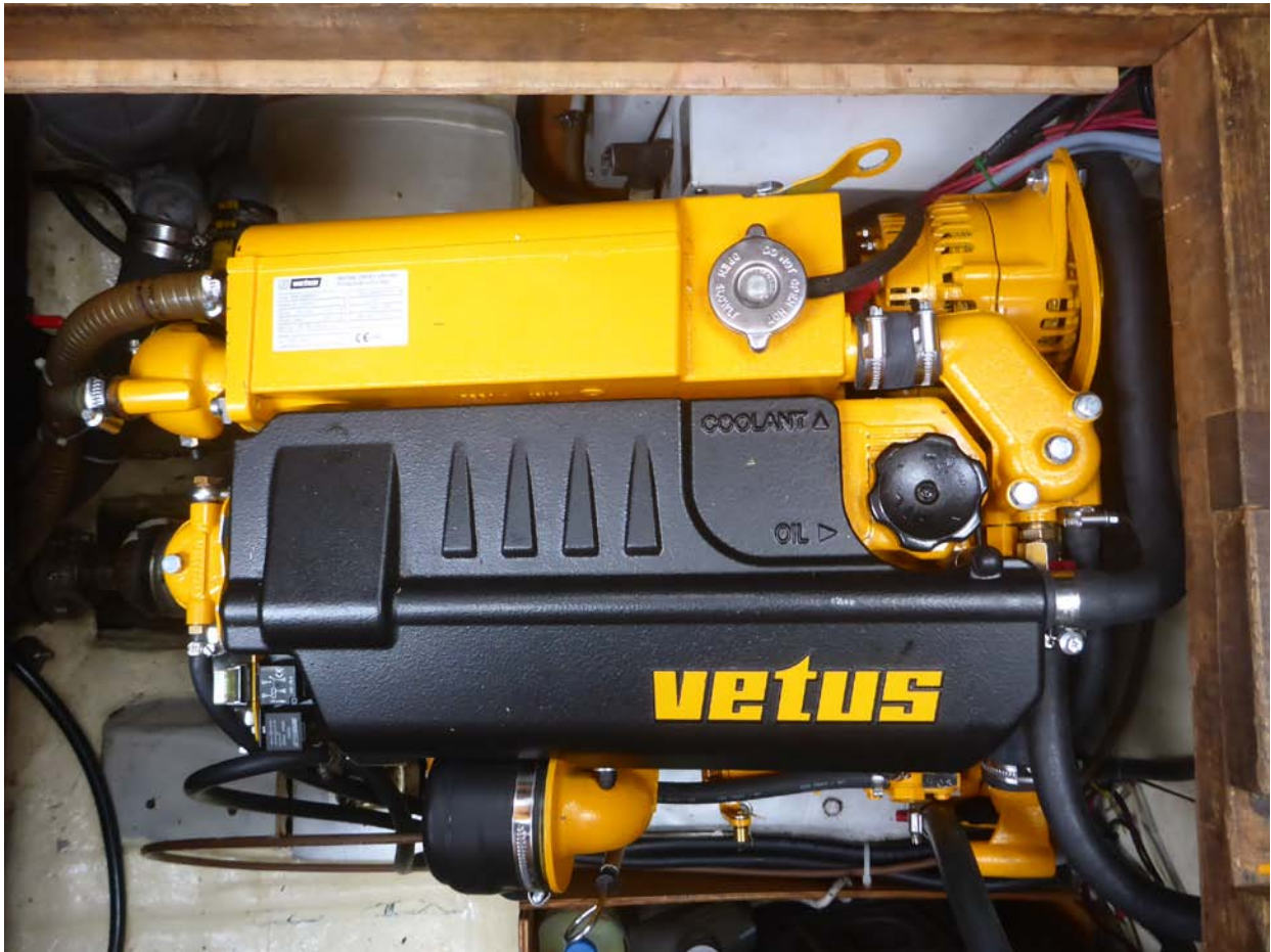
Figure 18 Top of motor: To the top is seen shiny lid for cooling liquid and to the lower right the black lid for the oil.
