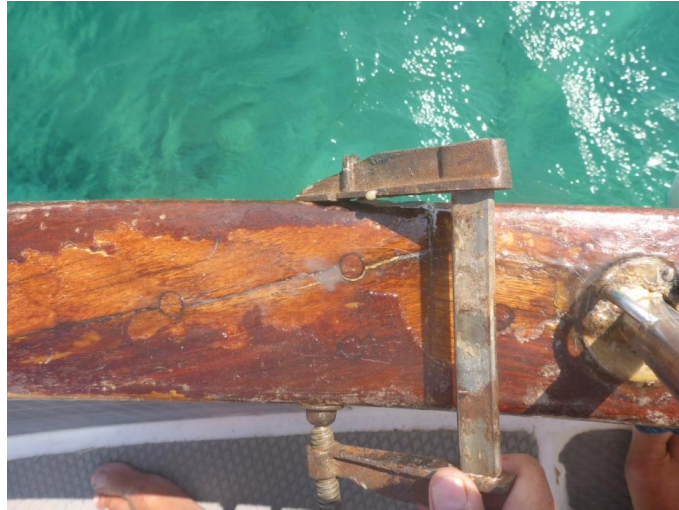
Jens repairs the wood which has split because of the sun ...
