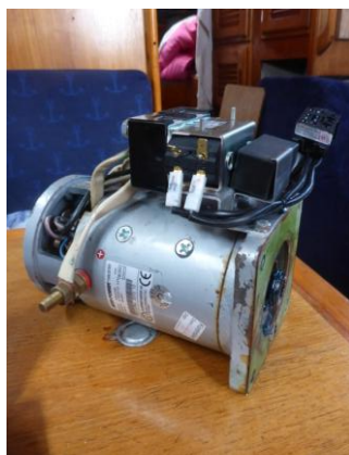
Jens takes out the bow-propeller engine
