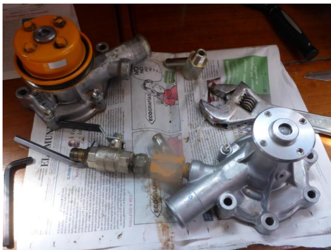
The old pump on the left, the new one on the right
