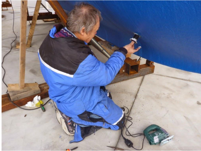
Jens is installing a new log
