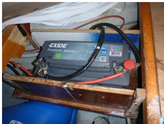
Left: Bow thruster batteries are under the plate. It is secured with a solid fuse of 400A and a switch: Right: front winch battery.
