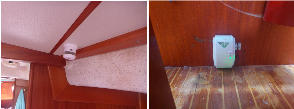
Gas detector (right) and smoke detector (left).
