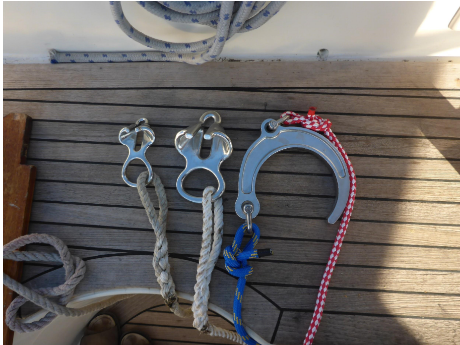
Anchor hooks for 6 and 10mm chain (left) and tool to untangle crossed anchor lines (right)..
