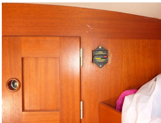
Automatic fuse for front winch.
