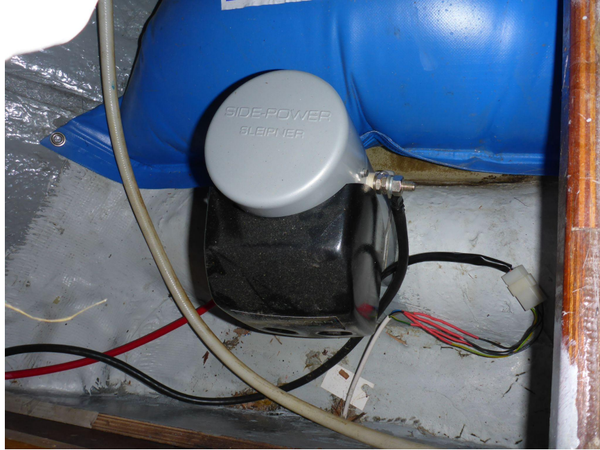
Bow thruster. In front is seen the flexible extra water tank.
