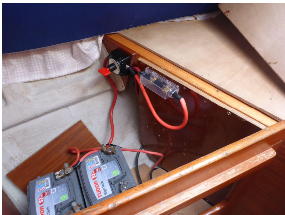
Left: Bow thruster batteries are under the plate. It is secured with a solid fuse of 400A and a switch: Right: front winch battery.
