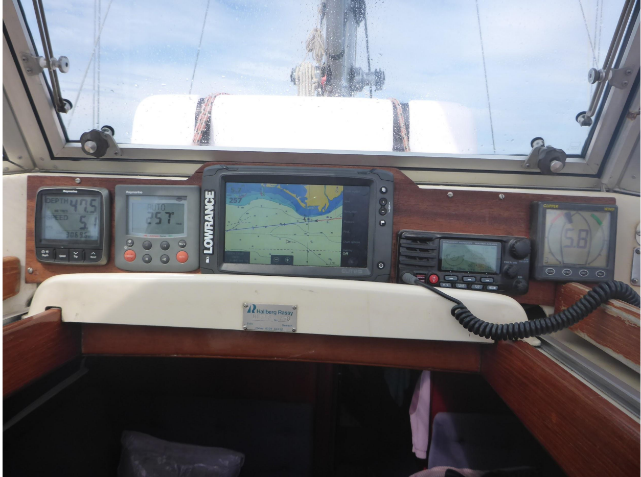
Instruments in the cockpit. From left: depth-speed, autopilot, plotter, VHF and wind.
